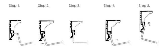
The same bracket is used for both under desk (top) and modesty panel fixing. If extra space is needed, for example to access sockets, the basket may be moved to position 5 whilst access is required.
