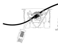
Angled data fascias allow data cabling to pass straight through PLATINUM, ensuring the integrity of cables which have a minimum bend radii (CAT5e, CAT6, etc)
