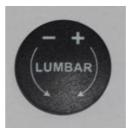
The right wheel adjusts the lumbar in and out of your spine by turning it clockwise or anticlockwise.
